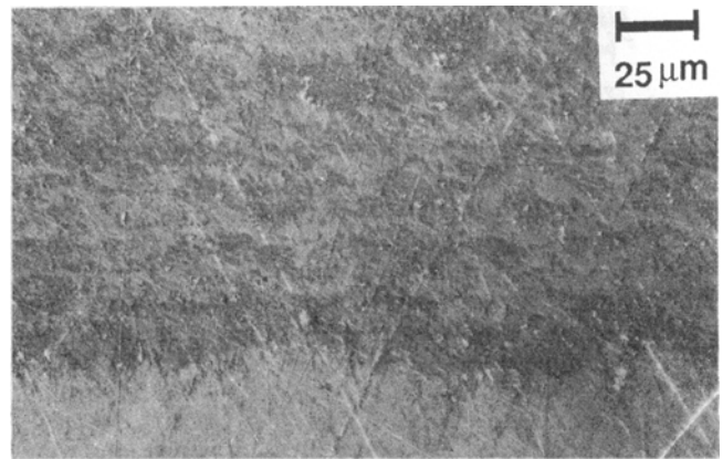
Fig. 1 Photomicrograph of WC/Co sample showing fine scratches before vibratory polishing. Compare with the final vibratory polished surface in Fig. 3.
